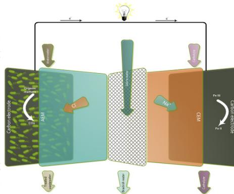
Figure 1. Microbial desalination cell MDC concept
